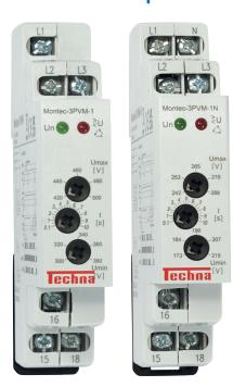
These relays monitor overvoltage, undervoltage, phase sequence and phase failure in 3 Phase AC systems. The Montec-3PVM-1 draws its supply from 3 live phases, which means that the relay remains functional even if one phase is lost. The Montec-3PVM-1N draws its supply from L1, L2, L3 and N, so the relay also monitors loss of the neutral.
